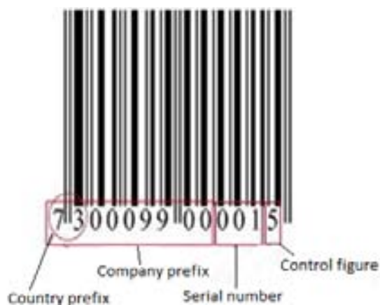
Figure 7. The construction of an EAN-13 code (Link 7).
